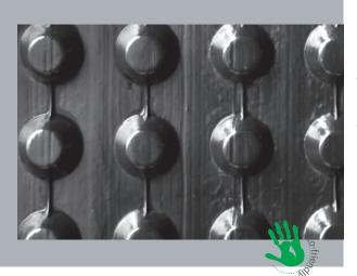
**PROJECT SPECIFICATIONS**: HDPE membranes are designed to protect waterproofing for retaining walls in integrated systems using BASIC and EXTENDER VERT membranes, laying polyester TNT as a separator and installing a drainage system (perforated pipe) to collect the water and channel it towards the drain.
